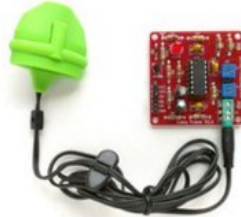
Easy pulse sensor based on photoplethysmog...
